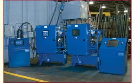
*Sorensen Systems designed and built three hydraulic power units and a PLC driven control system to remotely operate the gates from the passenger embarkation station on the San Antonio River Walk tourist attraction.*
