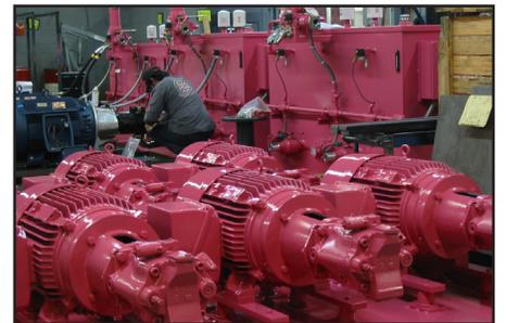
*Electric motors to power the hydraulic power unit are prepared for mounting onto a skid as final assembly is accomplished at Sorensen Systems headquarters.*
