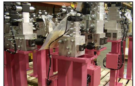
*Manifold assemblies installed as part of the hydraulic power units were also painted "pink", not for appearance, but for safety.*
